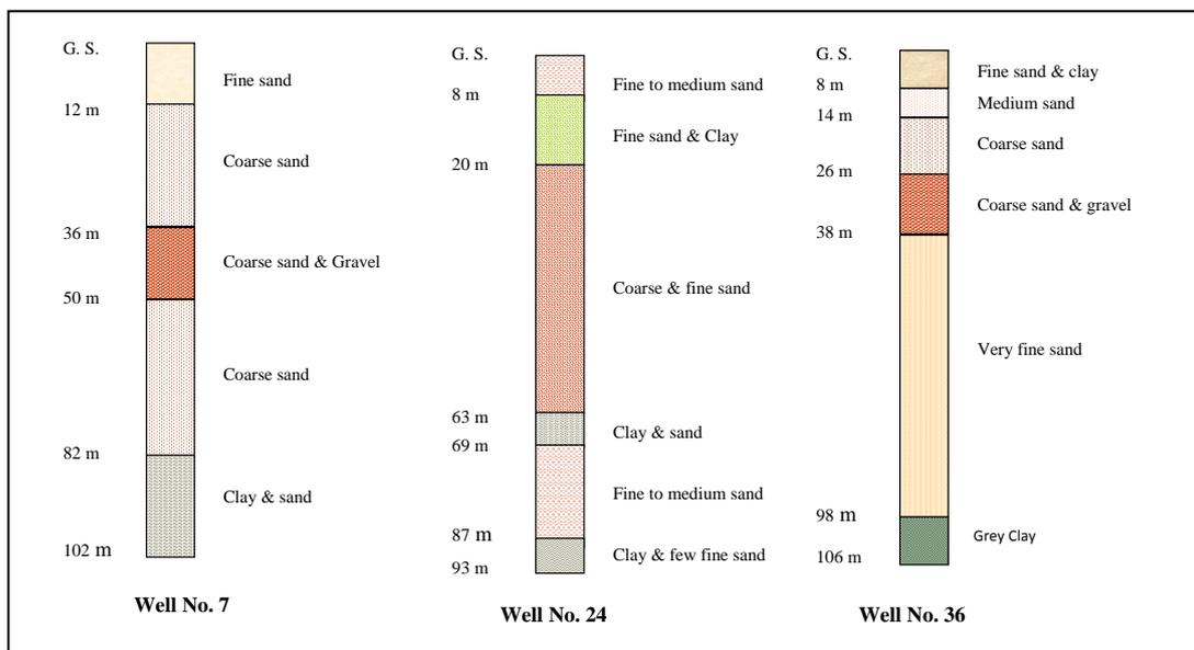
**Figure 2.** Geological map of Aswan and surrounding areas (Upper) and geological cross sections of the drilled wells at new Kima factory site (Lower), G. S. represents Ground Surface.
