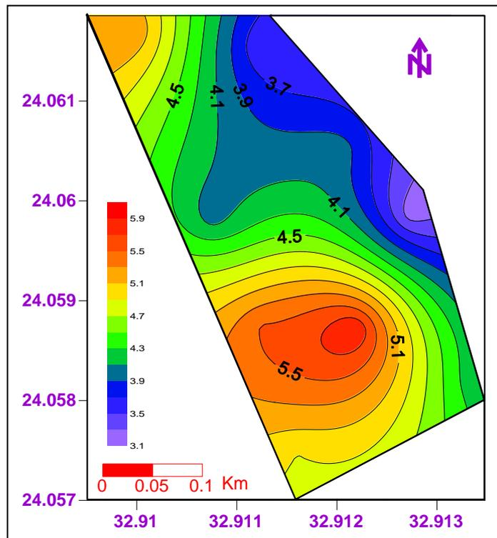
Figure 6. The amplification value over the factory's site.
